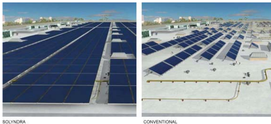
Figure 16 - Solyndra panels on left vs. conventional panels on the right.
